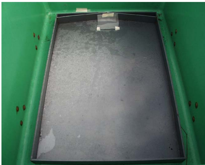
Figure 4 Above view of lysimeter. The inner container is shown which ensures leachate and runoff are kept separate.
