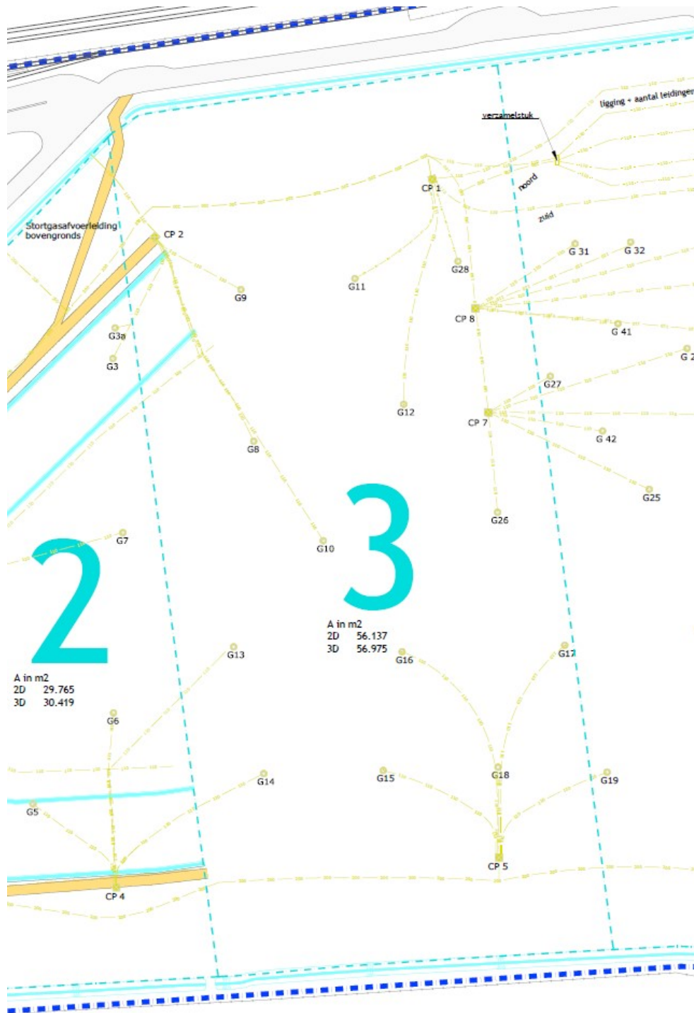
Figure 2: System for landfill gas recovery at compartment 3
